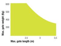
The shape, the height of the gate and the weather conditions can considerably reduce the values shown in the graph to the side. Use in windy areas 230Vac models.
