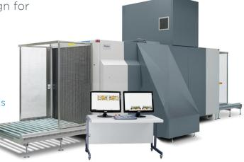
The Rapiscan 638DV is an advanced Dual-View X-ray system for screening of ULD, ISO standard, lower deck and large cargo pallet type freights. With a large and spacious tunnel size of 1,837 mm x 1,800 mm, Dual View technology and Automatic Explosives Detection feature, the Rapiscan 638DV is widely used for air cargo screening and customs applications where throughput is most important.
