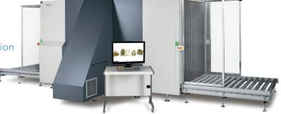
The Rapiscan 638XR is an advanced X-ray system for screening of ULD type, ISO standard, lower deck and large cargo pallet type freights. It has a high tunnel opening of 1,837 mm x 1,800 mm and uses innovative screening technology with automatic explosives and narcotics detection, to generate an outstanding high resolution view of the object under inspection.
