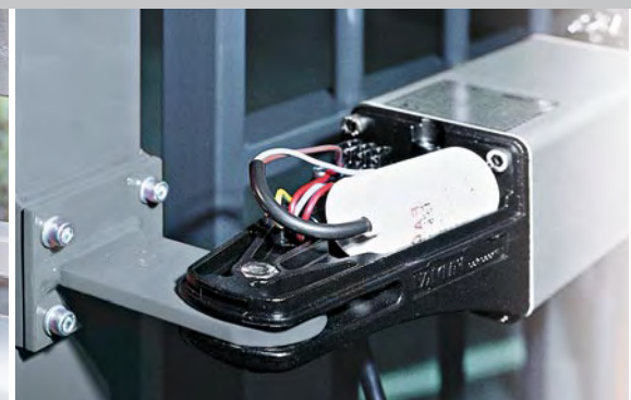
Capacitor fixed into place
